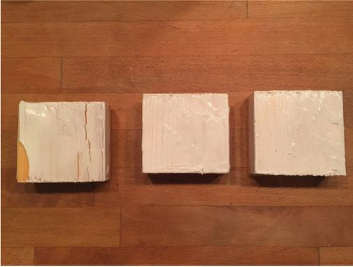
Abb. 1: Links: kein Harz, Mitte: 25%, rechts: 50% Harz-Zumischung. – Left: no resin, middle: 25%, right: 50% resin added.
